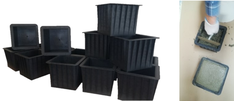
Figure 12 Moulds for concrete testing made of the rPP/NP composite.
