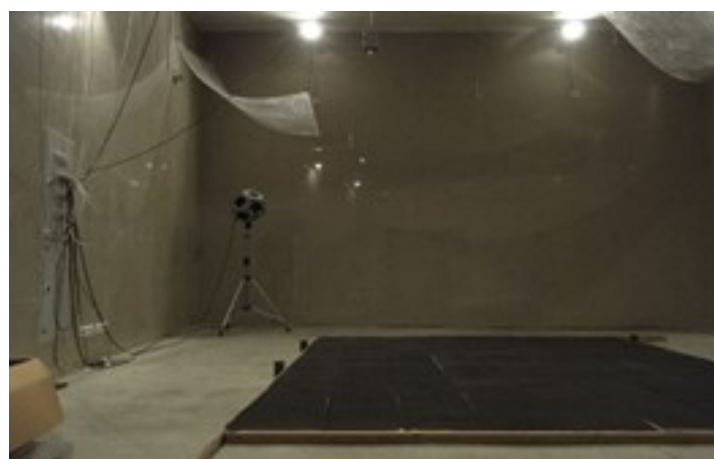
Figure 9 Reverberant sound chamber at the Building Research Institute (Instytut Techniki Budowlanej, ITB), used to measure the reverberant sound absorption coefficient \alpha_s in accordance with the PN-EN ISO 354 standard.
